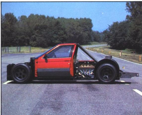
In line with existing Formula One design, the ProCar has a central 'tub' of aluminium/Nomex honeycomb, lined with carbon and kevlar. The longitudinally-mounted engine forms a fully stressed part of the chassis.
