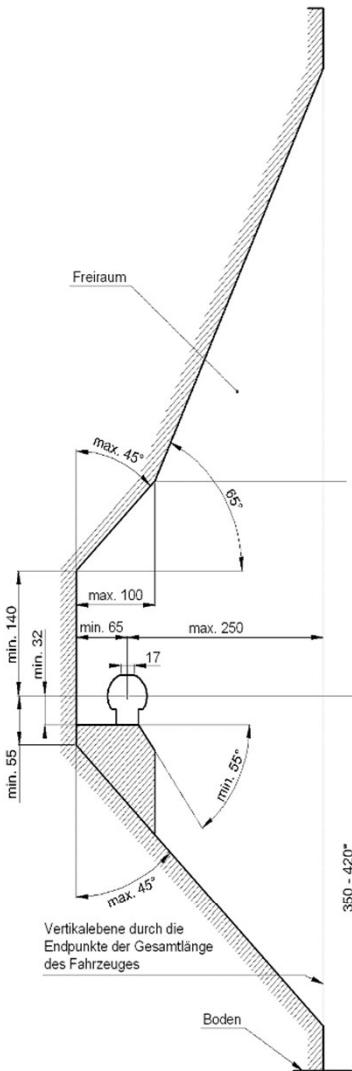
**EN** Make sure to provide clearance according to appendix 7, figures 25a and 25b of the ECE-R 55 regulations.
