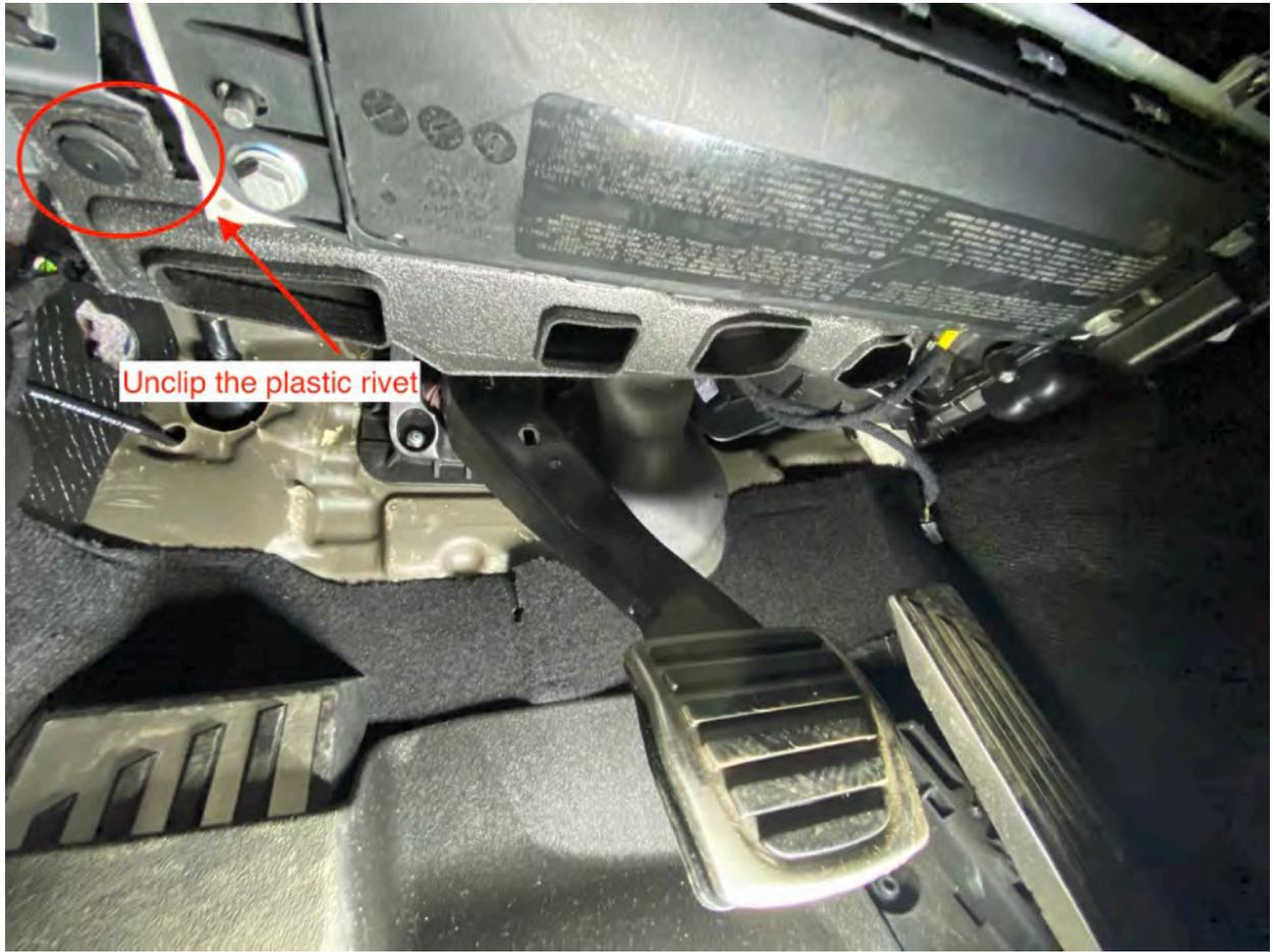
Unclip the plastic rivet
