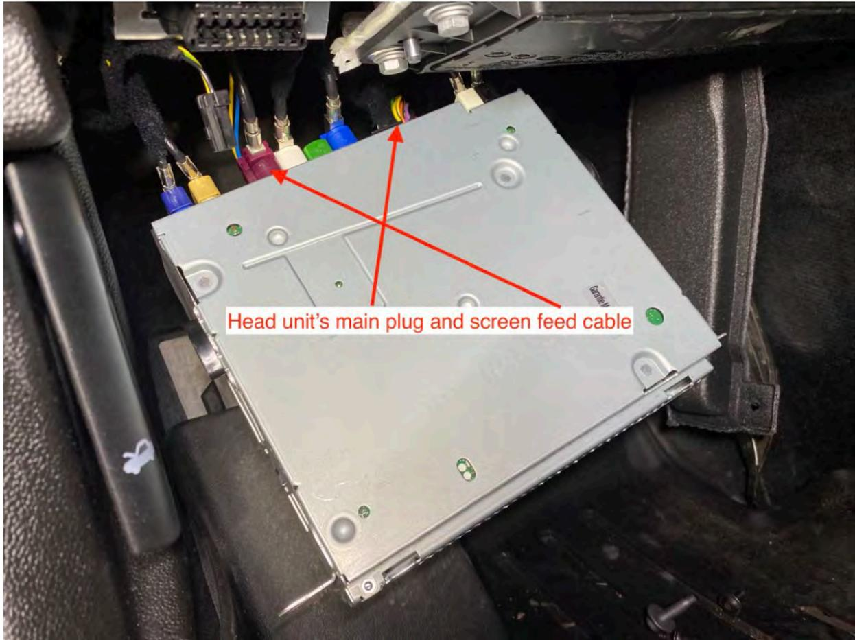
Head unit's main plug and screen feed cable
