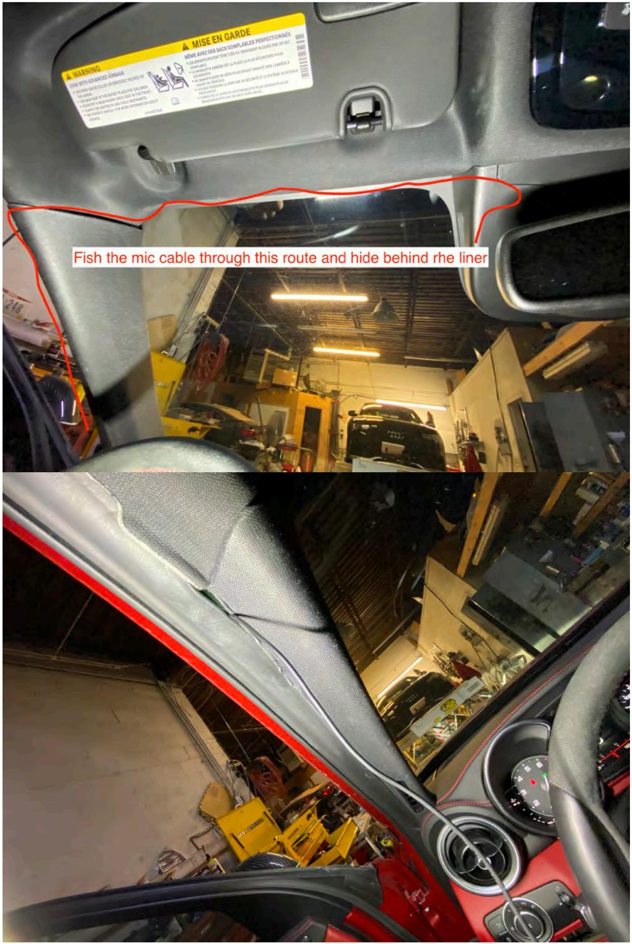
Fish the mic cable through this route and hide behind the liner
