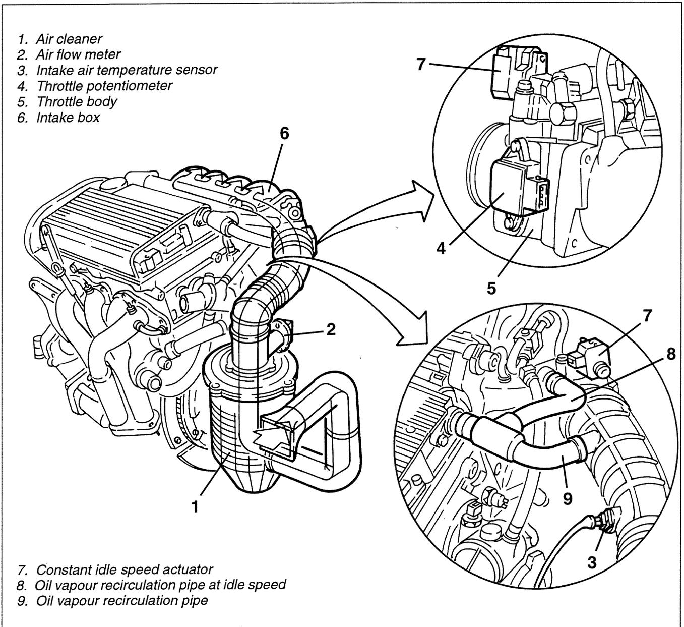
**NOTE:** From chassis no. .... the air supply system is fitted with intake resounders (for removing/refitting see specific paragraph).
