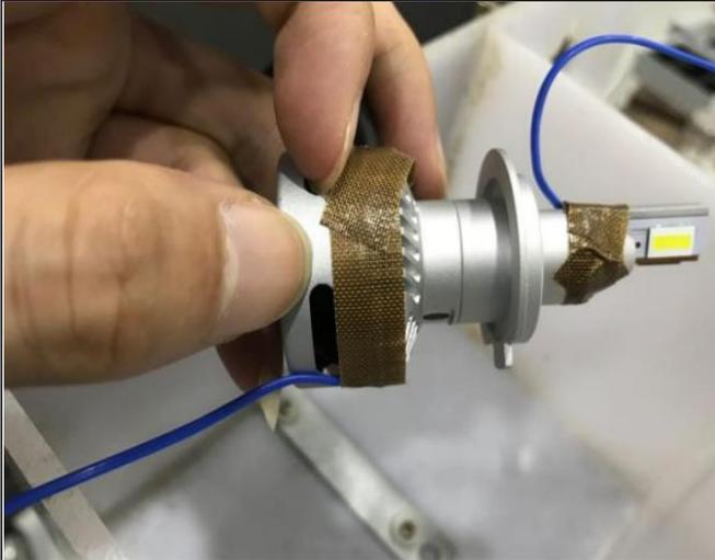
**T6** showed the working temp which is near the LED chip
