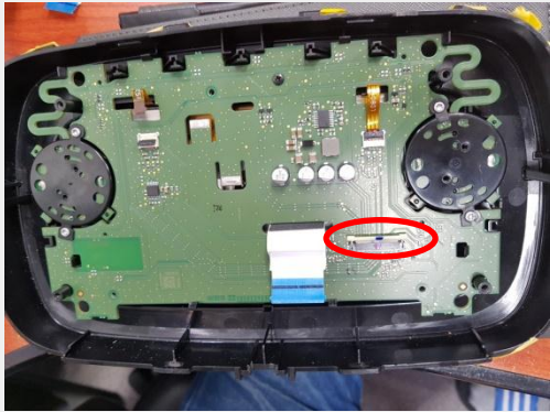
Remove the original FFC cable in a circle
