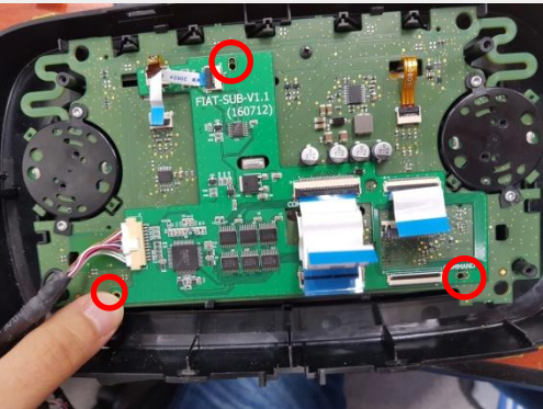
Put the supplied subboard on the top of PCB board and assemble bolts in marked places (Use OEM bolts)
