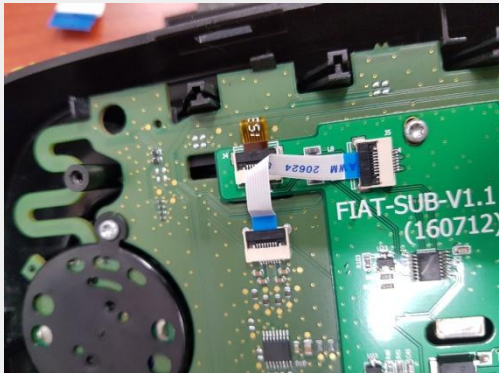
Connect touch cable as shown above
