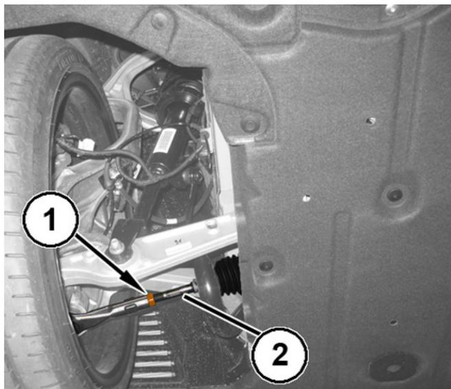
**NOTE:** When the adjustment is completed, the number of free threads on the right tie rod should be the same as the number of free threads on the left tie rod.
