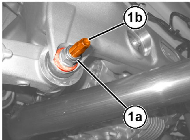
**NOTE:** After adjusting the rear camber angle, recheck the half toe-in and if necessary repeat the adjustment.
